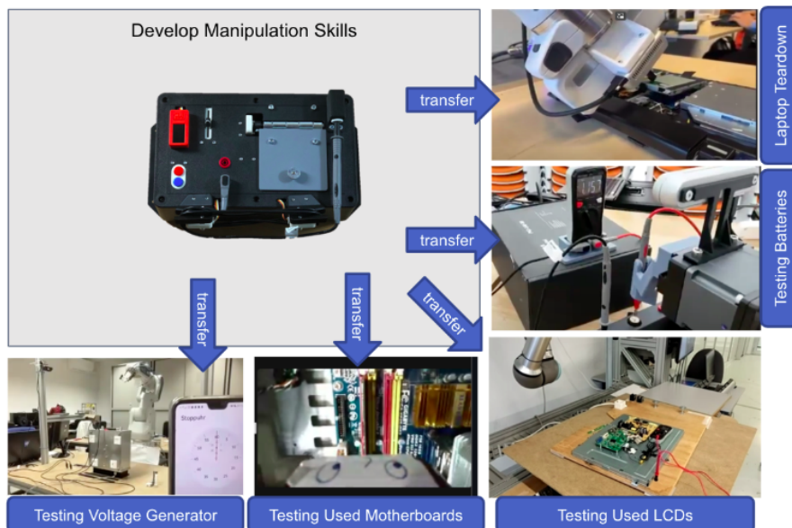
Figure 4.6: Examples of manipulation skill transferability demonstrations from the task board to real world applications.
